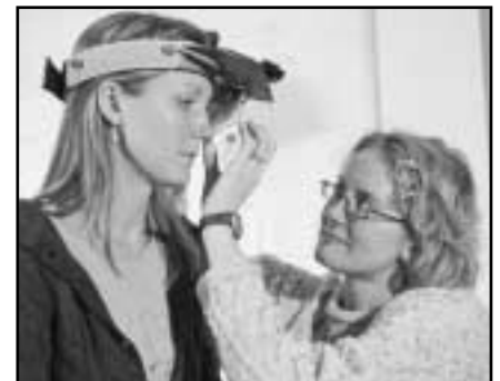
Prof. Lori Vallis, right, along with graduate student Catherine Lowrey, is using what's called a gaze monitoring system (pictured); to tell exactly where a participant is directing their visual gaze.
